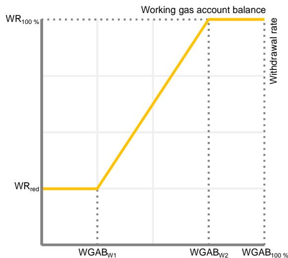
The maximally usable *withdrawal rate* is subject to the following characteristic restriction:
