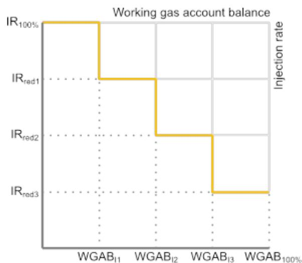
The maximally usable *injection rate* is subject to the following characteristic restriction:
