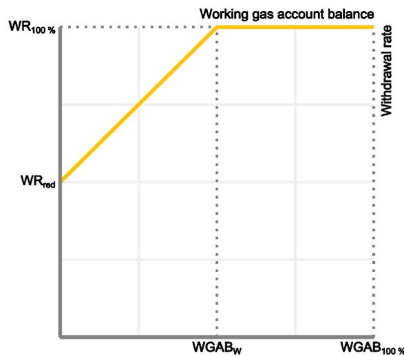
The maximally usable *withdrawal rate* is subject to the following characteristic restriction:
