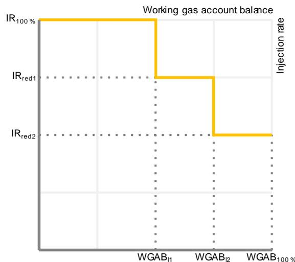
The maximally usable *injection rate* is subject to the following characteristic restriction:
